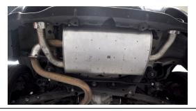
3 USING A 14mm, REMOVE THE BOLTS CONNECTING THE MIDPIPE TO THE CAT / OVERPIPE.
