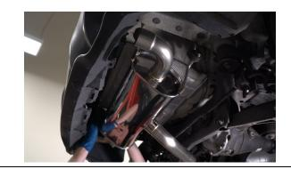
9 ROTATE PIPES AND FLANGES WHERE NECESSARY TO ENSURE ANGLES MATCH THE DIRECTION OF THE EXHAUST 11 INSTALL TIP CLAMP ONTO MUFFLER, THEN **INSTALL TIP.**
