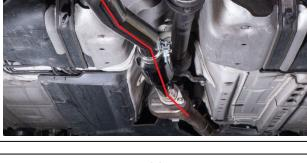
DUE TO MANUFACTURING AND SHIPPING, THE TIP MAY BE A TIGHT FIT ON THE EXHAUST PIPE, AND USE OF LIGHT FORCE MAY BE NECESSARY TO GET THE THEM IN THE PROPER POSITION. IF NEEDED, WE HIGHLY RECOMMEND A CLEAN RUBBER MALLET AND PADDING (SUCH AS A MICROFIBER TOWEL) TO LIGHTLY TAP THE TIP ONTO THE PIPE. THE TIPS ARE DESIGNED TO HAVE ~3/4" ADJUSTABLE VARIANCE IN THE DEPTH AND CAN BE SET TO YOUR TASTE 14
