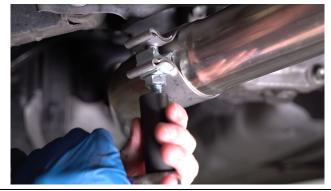
FIT THE TIPS TO DESIRED DEPTH AND **ORIENTATION, WHILE ENSURING THAT THERE** IS NO CONTACT WITH THE BUMPER
