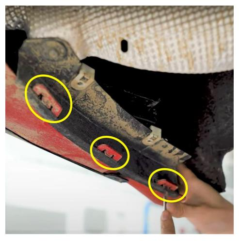
4 – Place a bolt through the holes opened earlier by the 2 clips. Ensure that both the bumper cover and black finger from the bumper valence have the bolt through them.
