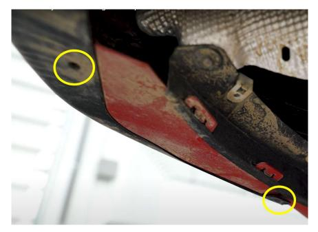
3 – Using a screwdriver or similar pry tool, release the 3 tabs securing the lower side of the bumper. Repeat on both sides.
