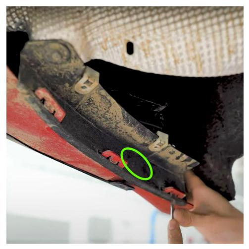
6 – Reinstall the bumper cover to the support bracket and engage the tabs.
