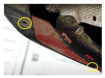
5 – Using a power drill and a drill bit, drill a 5/16 hole directly in front of the hole for the bolt installed in step 4 on the black bumper support. Use caution when drilling not to go through the bumper cover.
