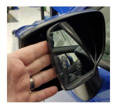
3 – Slide the glass down slightly to release the 2 hooks shown below in **Figure 1.** Then, if applicable, unplug the mirror heater wires and turn signal connections
