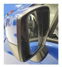
2 – Next put your hand behind the mirror glass and plastic frame that the glass is attached too and pry outward towards the bottom of the glass. This should release the 2 clips holding it in place.
